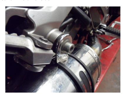
Rotate link pipes to obtain alignment and clearance. Starting from the front working rearwards, tighten all clamps and fasteners.
