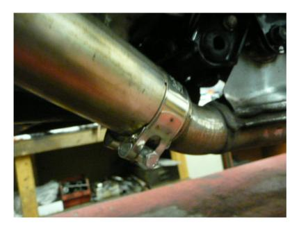
Fit silencer with 52/55mm clamp on to link pipe. Now fit strap onto silencer and to frame. Repeat on the other side.
