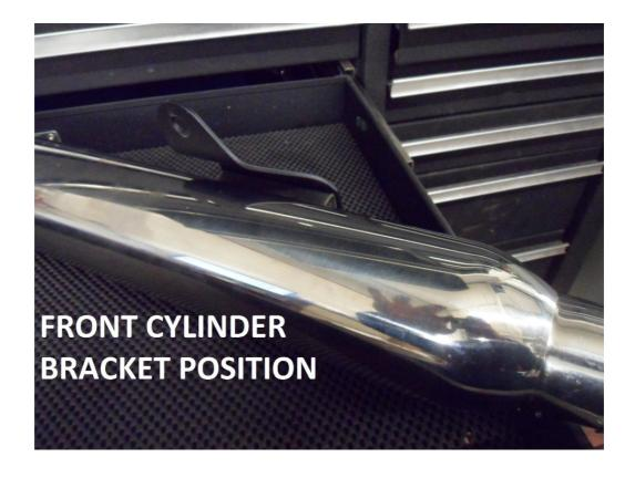
• Fit the front, lower silencer to the downpipe fully tightening the mounting bracket bolt, (arrowed).
