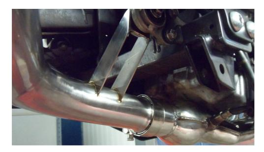
• Remove the pillion footrest pin and fit the mounting bracket using the cap screw.
