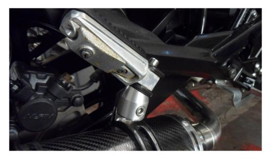
• Fit silencer with clamp on to the link pipe and fit the strap around the silencer and to the bracket.
