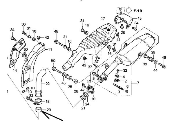
Clean collector pipe of old gasket material, dirt and carbon deposits.
