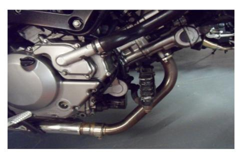
• Disconnect lambda sensor and remove standard silencer.
