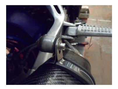
Rotate link pipe to obtain alignment and clearance.
