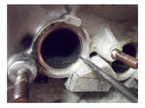
• Insert new cylinder port gaskets.
