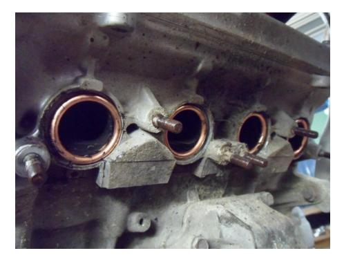
• Insert one pair of down pipes into the collector and the cylinder head.
