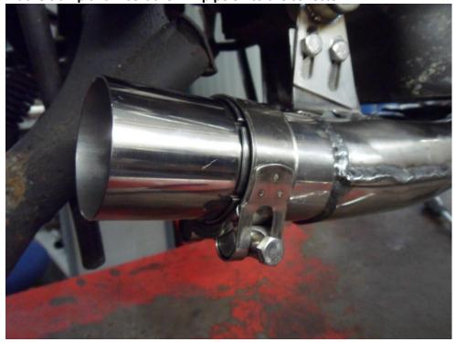
• Fit the OEM silencer with clamp on to the link pipe.
