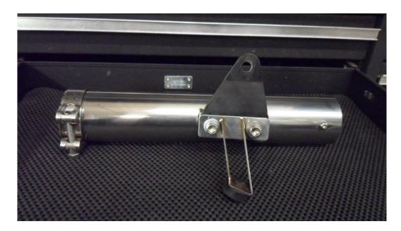
Attach the silencer to the collector and fit the spacer in between the frame and the silencer bracket.
