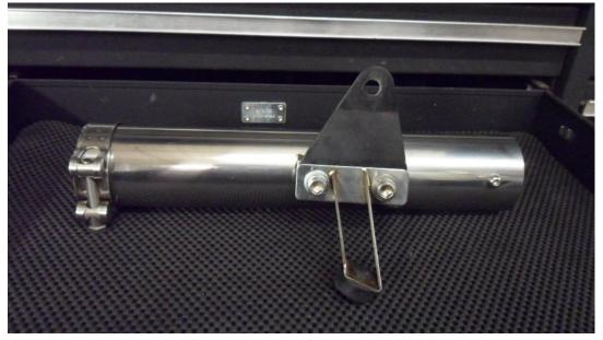
• Attach the silencer to the collector and fit the bracket behind the frame.
