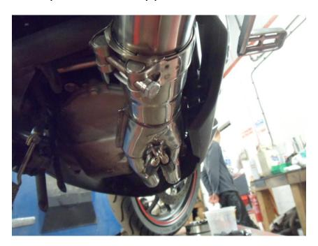
• Fit silencer with clamp on to the link pipe and fit the strap around the silencer and to the frame.
