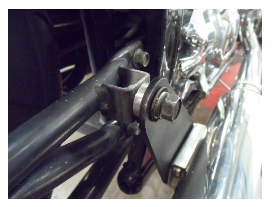
• Fit the rear, upper silencer bracket and spacer to the frame.
