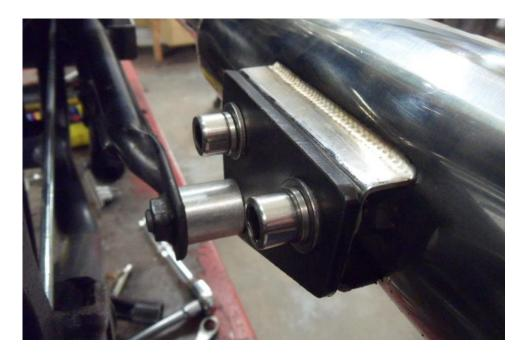
• Fit the rear, upper silencer to the downpipe and to the bracket.
