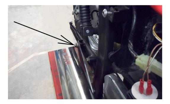
• Fit the rear, upper silencer to the downpipe fully tightening the mounting bracket.
