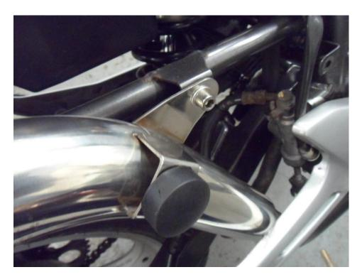
• Fit the silencer with clamp on to the link pipe and fit the strap around the silencer and to the spacer.
