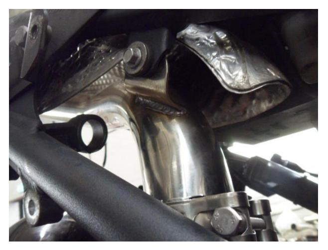
• Fit the secondary pipe to the frame.
