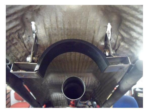
• Fit the silencer bracket to the frame.
