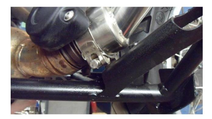
• Fit the silencer with clamp on to the link pipe and fit the strap around the silencer and to the bracket.
