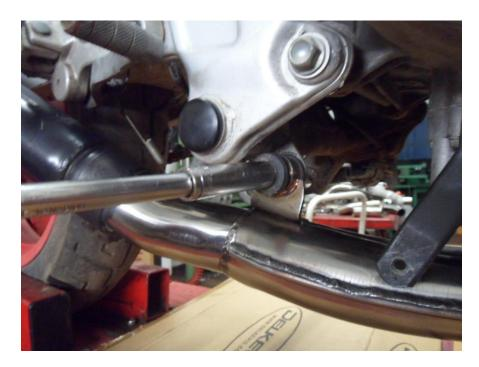
Tighten the cylinder head nuts and attach the springs.
