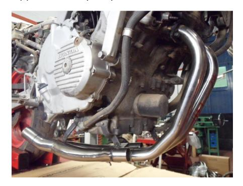
Insert pipes 1 and 4 into collector and into the cylinder head.
