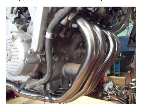
Fit lower mounting bolt and fully tighten.
