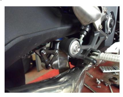
• Replace pillion footrest pivot pin with the 45mm cap screw.
