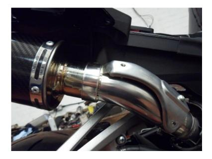
Insert silencer, note clamp goes over the heat shield.
