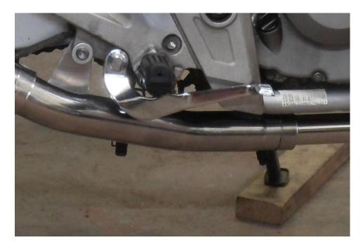
• Fit the silencer with clamp on to the link pipe and fit the strap around the silencer and to the bracket.
