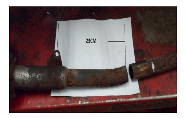
Clean the down pipe of dirt and rust deposits.
