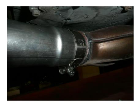
Fit dropdown bracket to the inside of footrest hanger. Fit silencer with clamp on to link pipe. Now fit strap onto silencer and to bracket.
