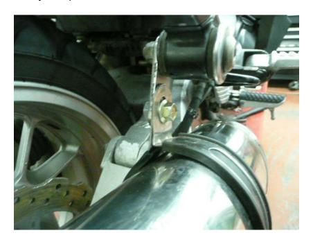
Rotate link pipe to obtain alignment and clearance.
