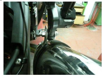
Rotate link pipe to obtain true alignment and clearance, and when you are happy, Starting from the front, tighten all clamps and fasteners.
