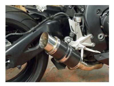
Now fit the strap onto the silencer and to the <u>outside</u> of the footrest hanger.
