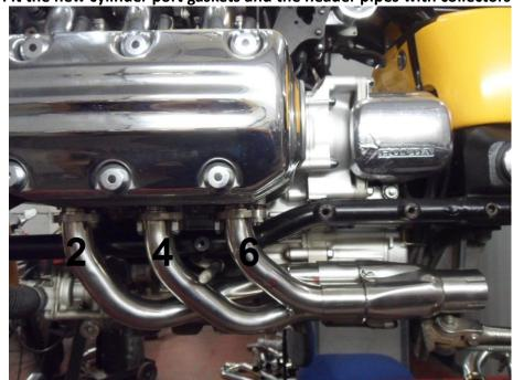
• Fit the new cylinder port gaskets and the header pipes with collectors finger tight.
