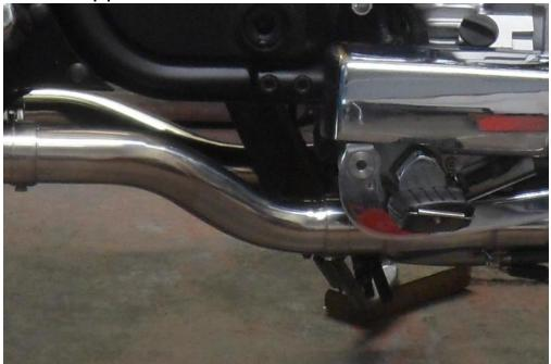
• Fit the mid-pipes into the collectors.
