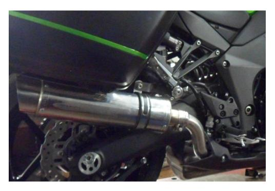
Starting from the front working rearwards tighten all clamps and fasteners. Start engine and check for leaks.
