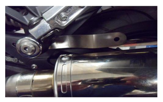
• Fit the strap around the silencer and to the bracket.
