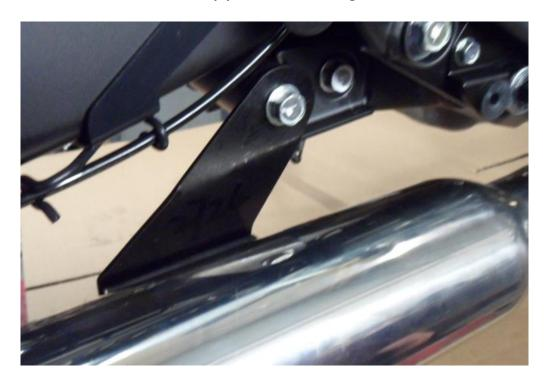
Attach the ABS wire heat shield on to the swing arm.
