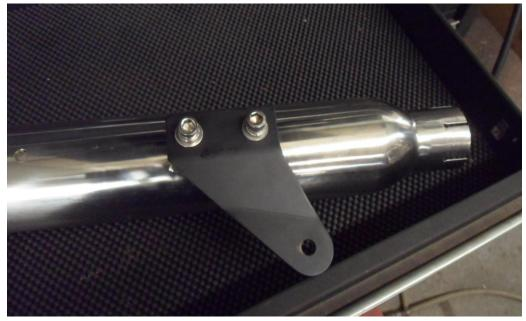
• Fit the silencer to the header pipe outlet, attaching the bracket to the frame.
