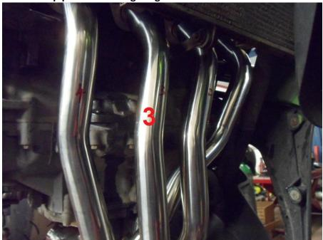
• Fit the clamp and insert the link pipe on to the collector attaching to the frame.
