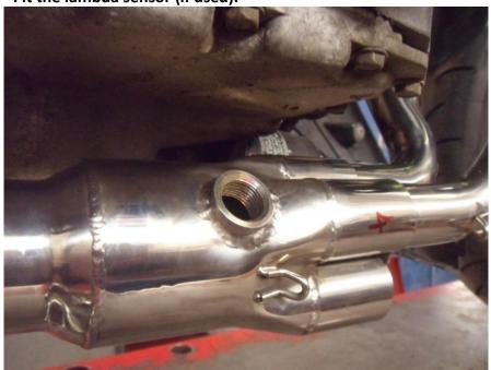
• Fit header pipes 2 and 3 finger tight.
