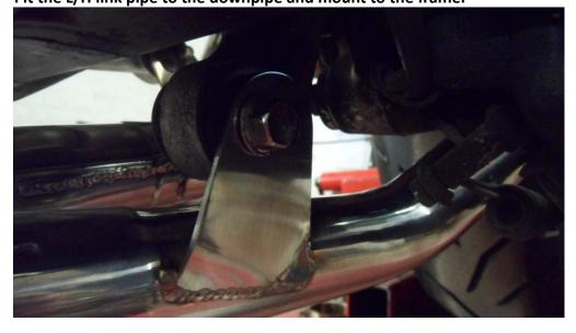
Remove the pillion footrest brackets and re fit with the silencer mounts and spacers.
