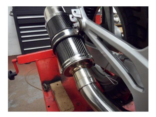
Rotate link pipe to obtain alignment and clearance. Starting from the front, tighten all clamps and fasteners.
