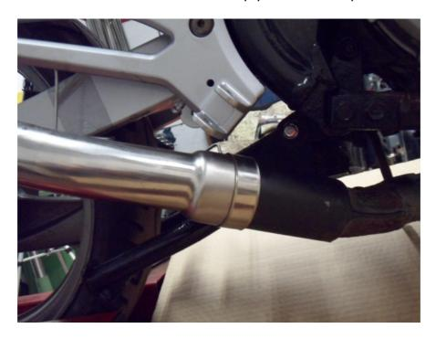
Fit silencer with clamp on to link pipe. Now fit strap onto silencer and to frame.
