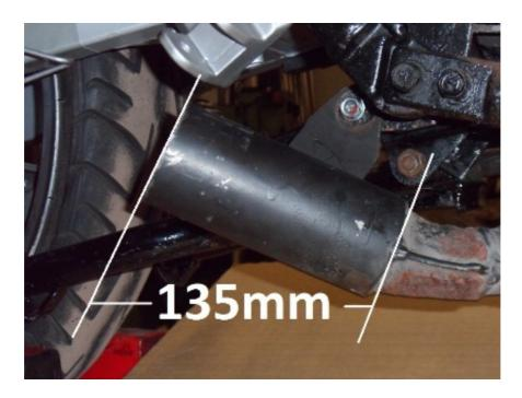
De burr the outlet end and fit link pipe with clamp.
