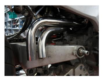
Insert middle pipes into collector.
