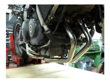
4. Fit collector link pipe, aligning stand stop and fit standard silencer.
