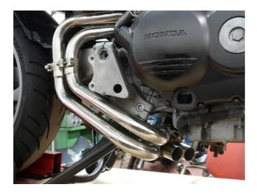
3. Fit cable bracket in between exhaust and frame, important that you do this correctly.
