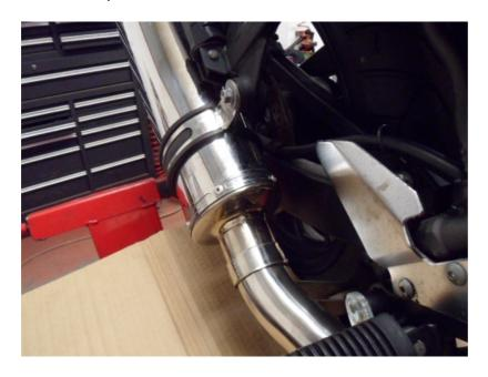
Rotate link pipe to obtain alignment and clearance. Starting from the front, tighten all clamps and fasteners.
