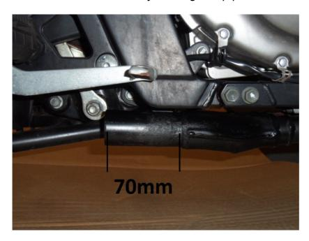
De burr the outlet end and insert link pipe with clamp.
