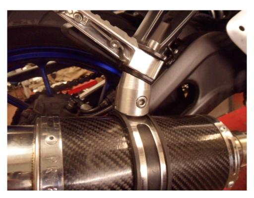
• Fit silencer with clamp on to the link pipe and fit the strap around the silencer and to the bracket.
