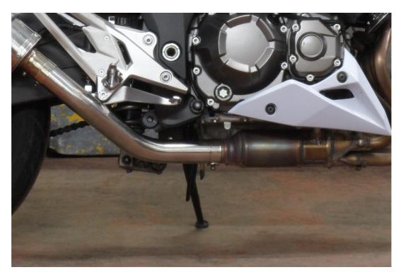
• Fit the silencer with clamp on to the link pipe and fit the strap around the silencer and to the footrest bracket.
