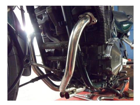
• Fit the inner down pipes.
