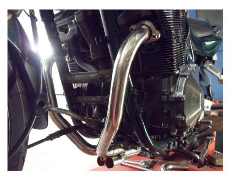
• Fit the inner down pipes.
