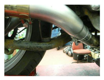
Nip up bolt, not too tight for now, just to support it. Remove footrest pin and replace with Allen bolt and Bracket.
