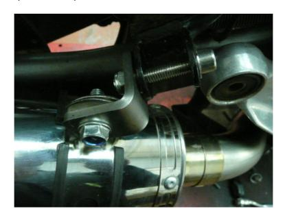
Smear a light coating of sealant inside silencer and fit with clamp on to link pipe.
