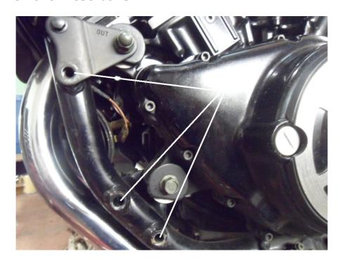
• Fit the L/Hand engine bar using the supplied Delkevic hardware.
