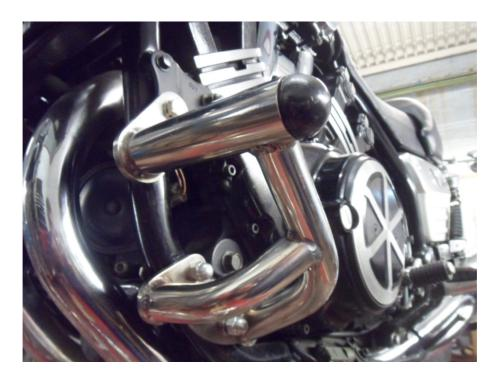
• Repeat on the R/hand side using the frame spacer.
