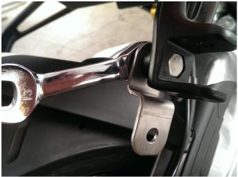
Fit new offset stainless steel hanger bracket onto the Hex head bolt as
