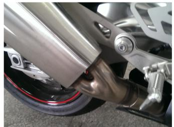
We recommend that the OEM silencer TORX bolt and washer (circled) are refitted to the original position and secured with the new M8 nyloc nut and plain washer supplied.
