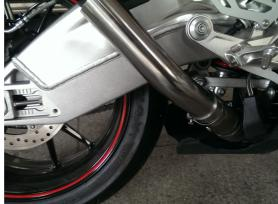
Apply a thin film of high temp sealant to the inlet of the silencer and fit silencer to the link pipe ensuring that the clamp is loosely fitted to the inlet side of the silencer. Slide "b" shaped silencer hanger and rubber over the silencer and align to the offset hanger bracket. Do NOT tighten any fittings at this stage.
