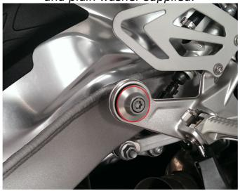
Remove R/H Pillion footrest and retain ALL of the parts for later refit. Fit new M8 Stainless Steel Hex Head bolt through the footrest hanger.
