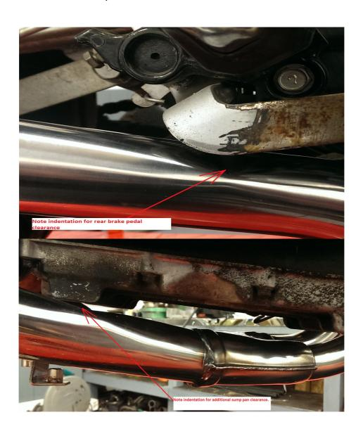
Once satisfied that the stand stop is in the correct position (see image below) and that there is clearance all around the exhaust, begin to tighten all clamps and fasteners starting from the front and working rearwards.
