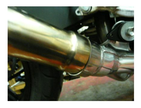
• Fit the silencer with clamp on to the link pipe and fit the strap around the silencer and to the bracket.
