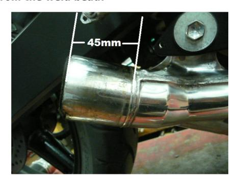
• De-burr the outer edge of collector pipe
