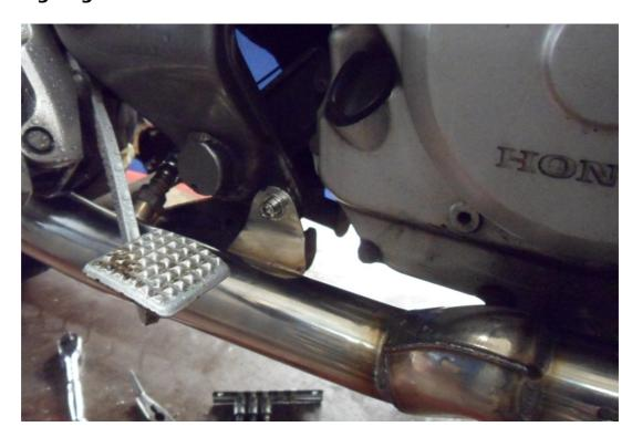
Fit the strap around the silencer and attach the mounting bracket loosely.
