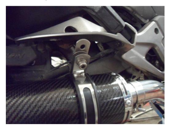
• Insert the bracket to the frame.
