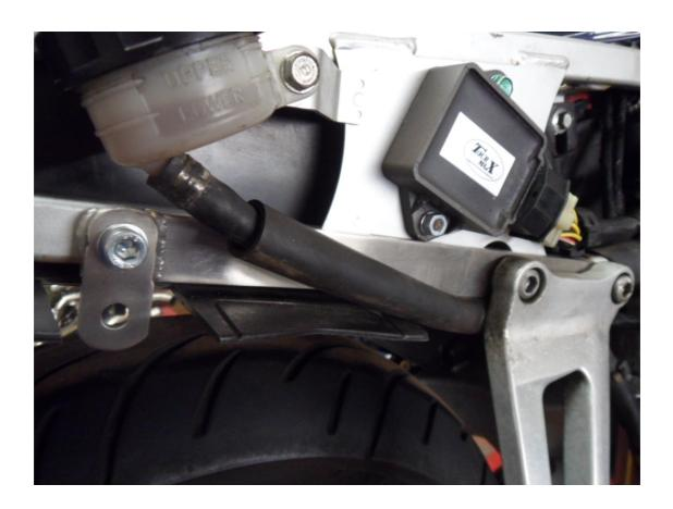
• Fit the link pipe to the OEM collector loosely at this moment.
