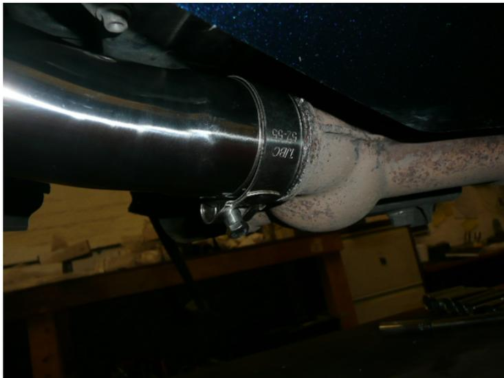
*Smear a light coating of sealant inside silencer and fit with clamp on to link pipe.*
