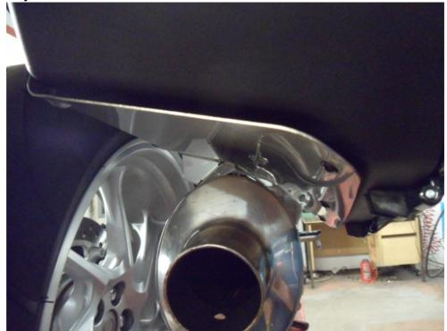
• Starting from the front, working rearwards tighten all clamps and fasteners.
