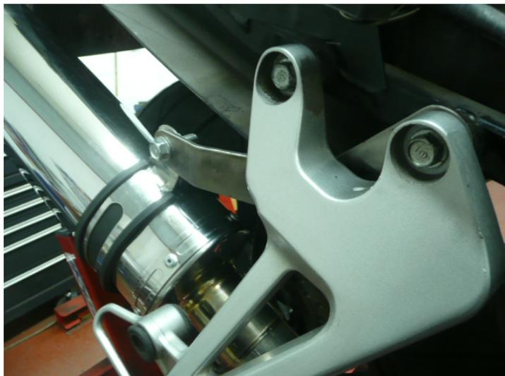
*Rotate link pipe to obtain true alignment and clearance, when you are happy, starting from the front, tighten all clamps and fasteners.*
