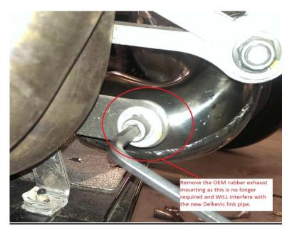
Apply a thin film of high temp silicone sealant to the outlet of the OEM downpipe and fit new Delkevic link pipe and clamp to the downpipe outlet but do **NOT** tighten the clamp at this stage.
