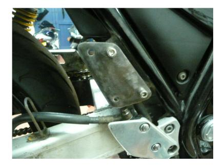
• *Refit footrest hangers using cap screws, nuts and washers.*
