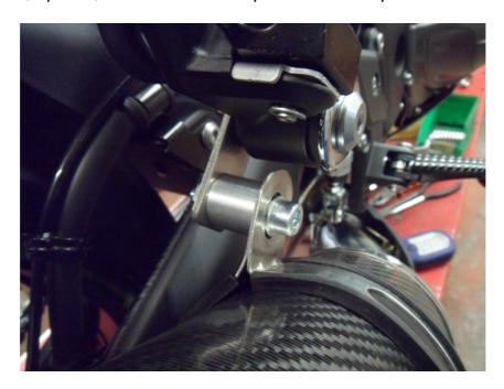
Fit the L/H side and then rotate the pipes to obtain alignment and clearance.
