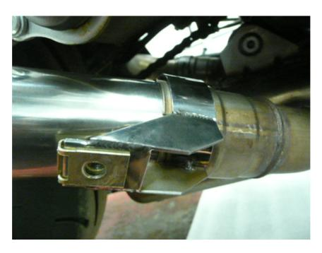
Insert the <u>longest</u> link pipe into R.H collector. Nip up bolt, not too tight for now just to support the pipe.
