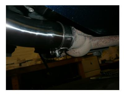
Insert silencer with clamp on to link pipe. Now fit strap onto silencer and to frame.
