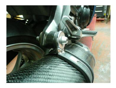
Repeat on the other side. Rotate link pipes to obtain alignment and clearance. Fully tighten all clamps and fasteners. Start engine and check for leaks. After your first ride out, check all fasteners for tightness, especially the baffle bolts.
