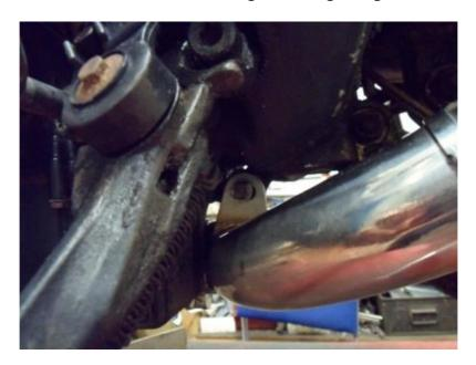
Insert new carbon gaskets inside slotted end of link pipes. Fit correct Clamps and insert on to the outlet.
