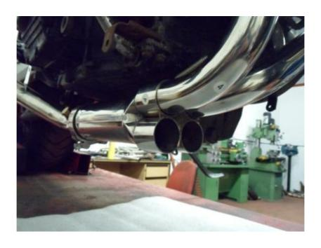
Now insert pipes 2 and 3 loosely. Twisting collector as required and fit the springs above and below.
