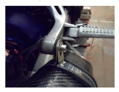
Rotate link pipes to obtain alignment and clearance. Starting from the front, tighten all fasteners and clamps. Start engine and check for leaks. After your first ride out check all fasteners for tightness.
